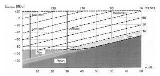
Figure 3: Dynamic range of a combination analogue microphone / preamplifier
